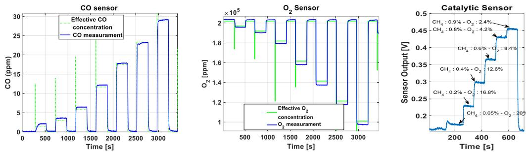
Figure 4 – CO and O<sub>2</sub> electrochemical sensor tests and catalytic sensor test with methane.
