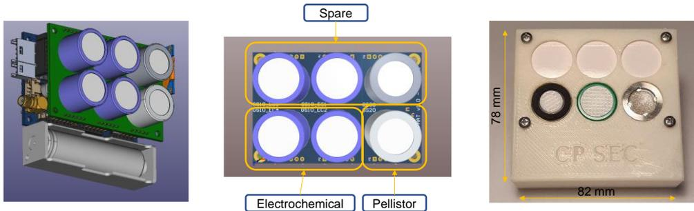
Figure 2 - 3D renderings and a photo of the internal structure and an enclosure of the sensor node.
