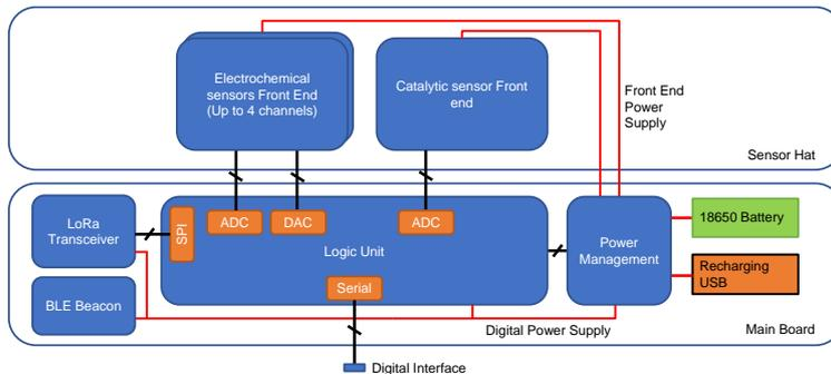
Figure 1 – Sensor node structure.
