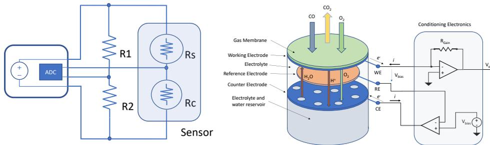
Figure 3 – (left): Conditioning electronics for catalytic sensors. (right): Conditioning electronics for electrochemical sensors.
