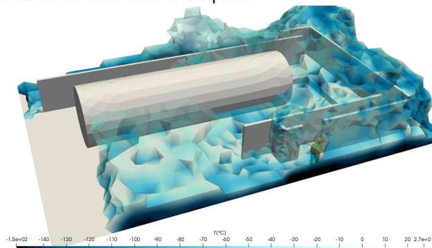
Figure 5: Temperature of LNG vapour in case 2
