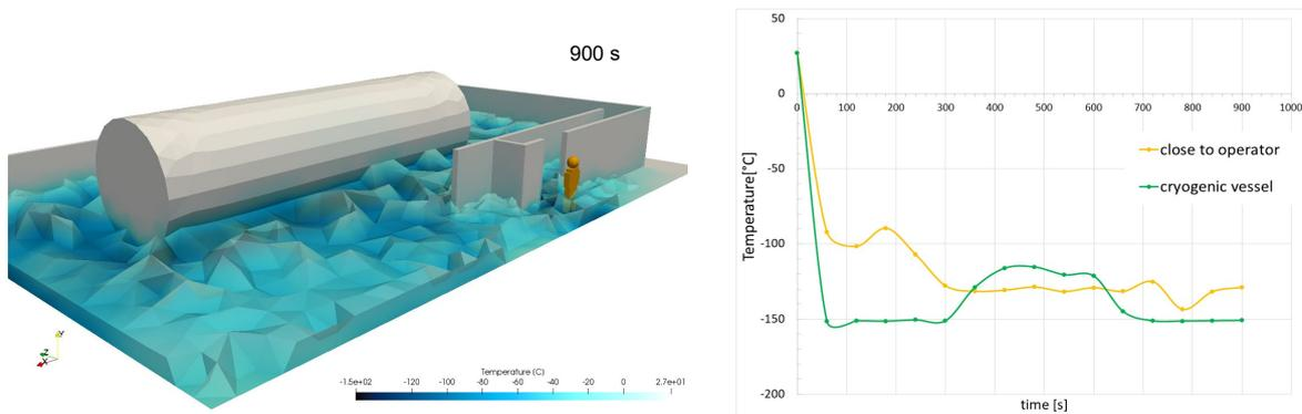
Figure 4: Temperature achieved close to operator (orange) and at cryogenic vessel (green) in case 1
