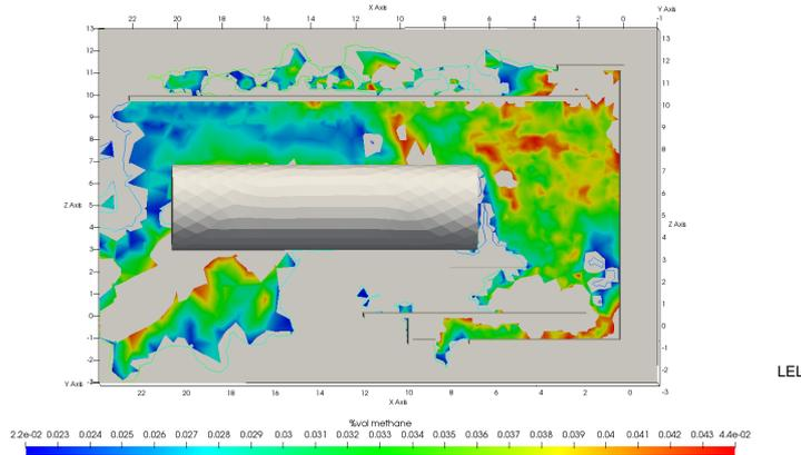
Figure 6: Concentration of methane in process area
