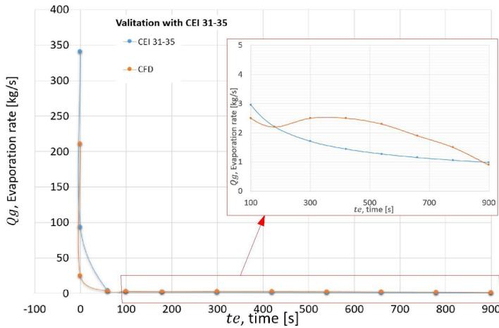
Figure 3: Comparison of results obtained with CEI 31-35 and CFD
