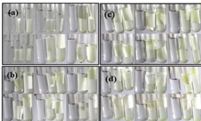
Figure 3: Test tubes showing solutions of (a) Ferrous Ammonium Sulfate (b) Potassium Dichromate (c) Cadmium Sulfate (d) Lead Nitrate with increasing concentrations (0.05, 0.1, 0.25, 0.5, 0.75, 1 ppm) respectively. The pH of each solution was also increased using an ammonia-water solution. Each test included a control (solution without paper strip) and two replicates for each concentration.
