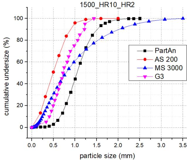
Figure 2: Analysis of the particle size distribution results under different measurement methods (sample: 1500\_HR10\_HR2)
