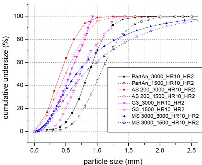
Figure 3: Comparison of the cumulative undersize of sample HR10\_HR2 at rotor speeds of  $1500 \text{ min}^{-1}$  and  $3000 \text{ min}^{-1}$  by different analysis methods
