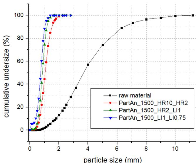
Figure 1: Particle size distribution of the raw material before and after milling at different parameters, as analysed by PartAn 3D
