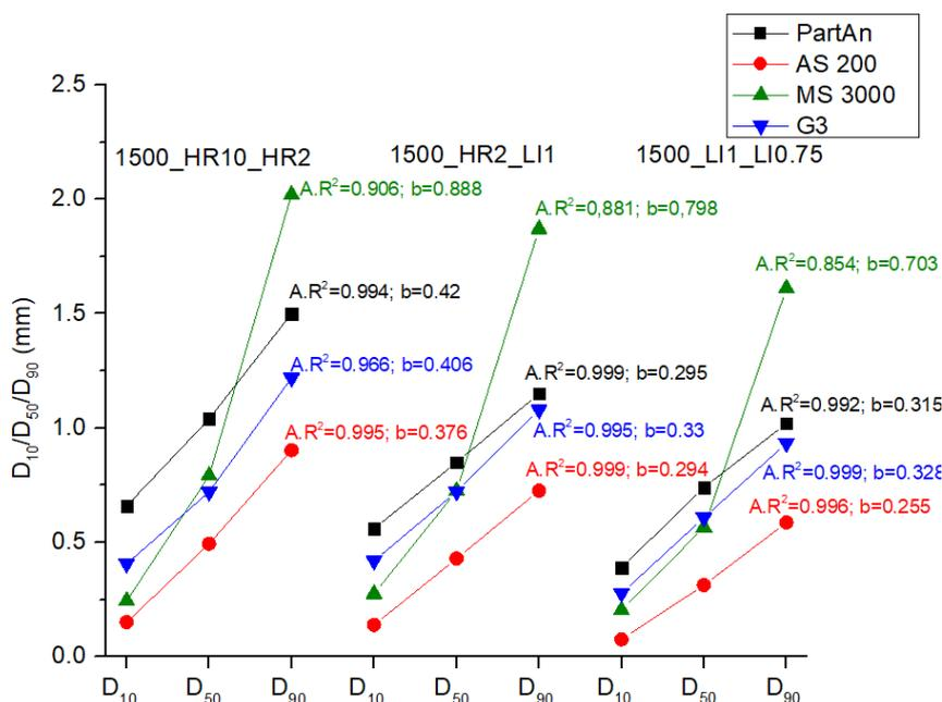
Figure 4: Particle size distribution presented by  $D_{10} - D_{90}$  for samples: 1500\_HR10\_HR2, 1500\_HR2\_LI1 and 1500\_LI1\_LI0,75 with statistical indicators
