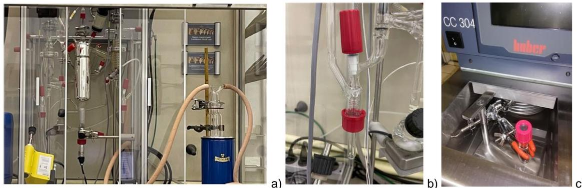
Figure 1: Pictures of: a) the Fischer Labodest VLLE 602 unit; b) one of the two receivers of the Fischer Labodest VLLE 602 unit; c) the thermostatic bath used for LLE measurements and the support properly designed to submerge the EC in it
