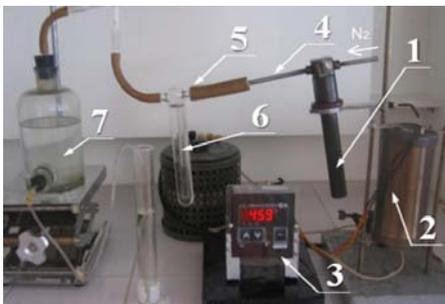
Figure 1: Laboratory setup for slow pyrolysis
