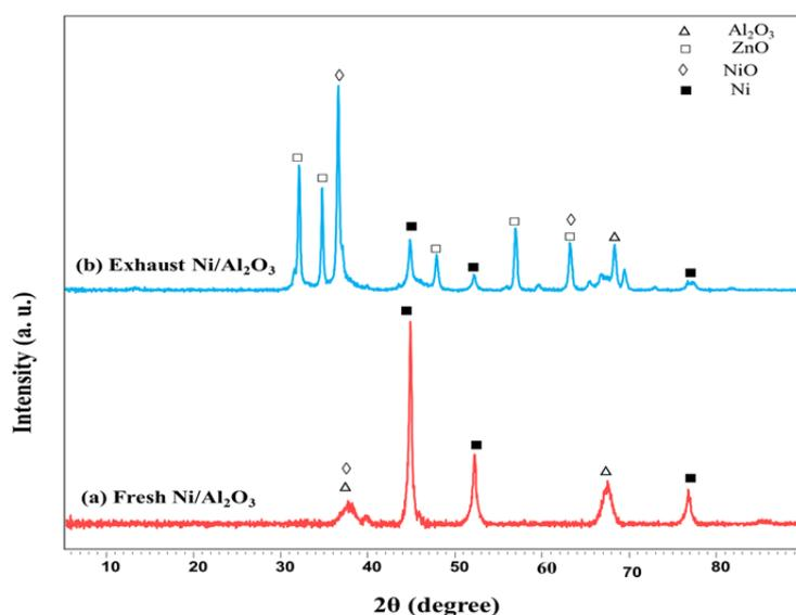
Figure 1: XRD patterns of fresh and exhausted Ni/Al<sub>2</sub>O<sub>3</sub> catalyst
