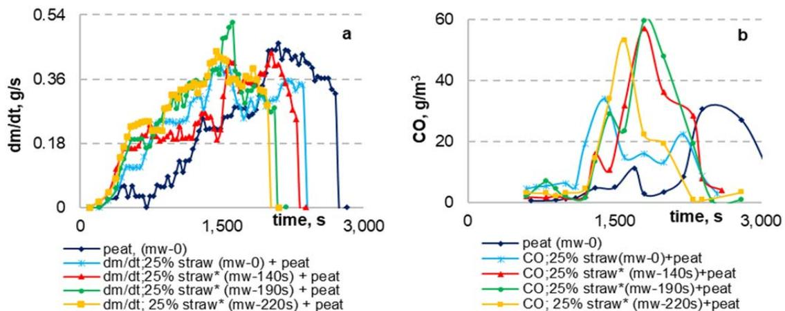
Figure 3: Effect of the increasing irradiation time for wheat straw pellets on the weight loss at the thermal decomposition of the 25% straw (MW)\*+peat mixture (a) and on the yield of CO (b)
