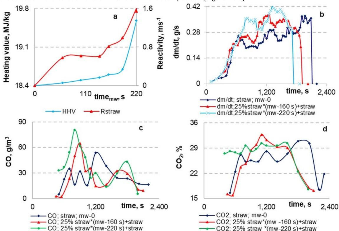
Figure 1: Effect of the duration of wheat straw pellets mw irradiation on (a) the heating value and reactivity of straw pellets; (b) on the weight loss rate, and (c, d) on the yield of volatiles during thermal decomposition of a mixture of MW pre-treated and raw straw pellets
