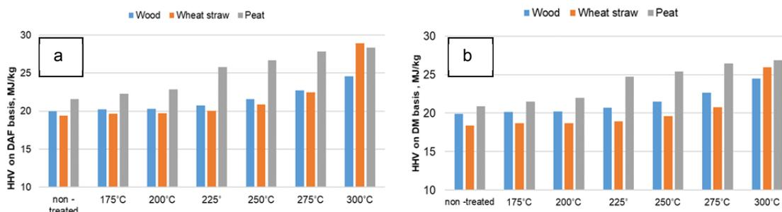
Figure 3: The HHV of non-treated and torrefied biomass samples recalculated on a dry ash-free (DAF) and DM basis
