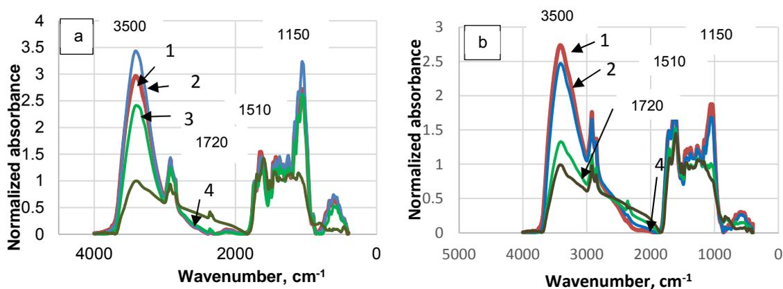
Figure 5: FTIR spectra of wheat straw (a), and peat (b) normalized at 1510 cm<sup>-1</sup>: non-treated (1), and torrefied at the temperatures: 200 °C (2); 250 °C (3), 300 °C (4)
