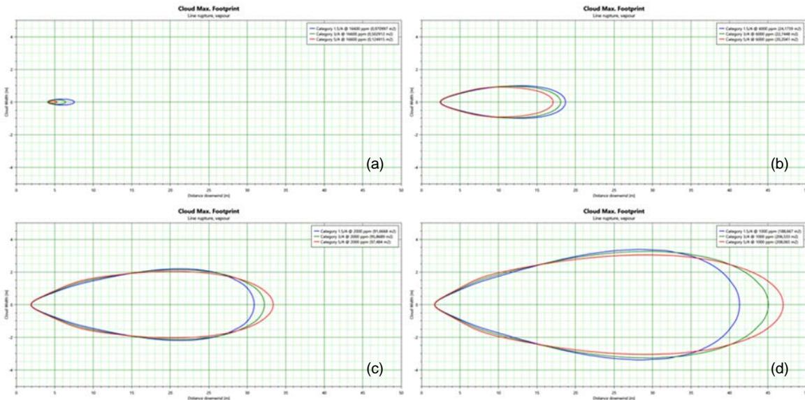
Figure 3: CO<sub>2</sub> iso-concentrations as a function of distance downwind at different values of CO<sub>2</sub> concentration (16,600 ppm (a), 6,000 ppm (b), 2,000 ppm (c) and 1,000 ppm (d)) after the breakage of a pipe leaving the extractor (Category of atmospheric stability: A)
