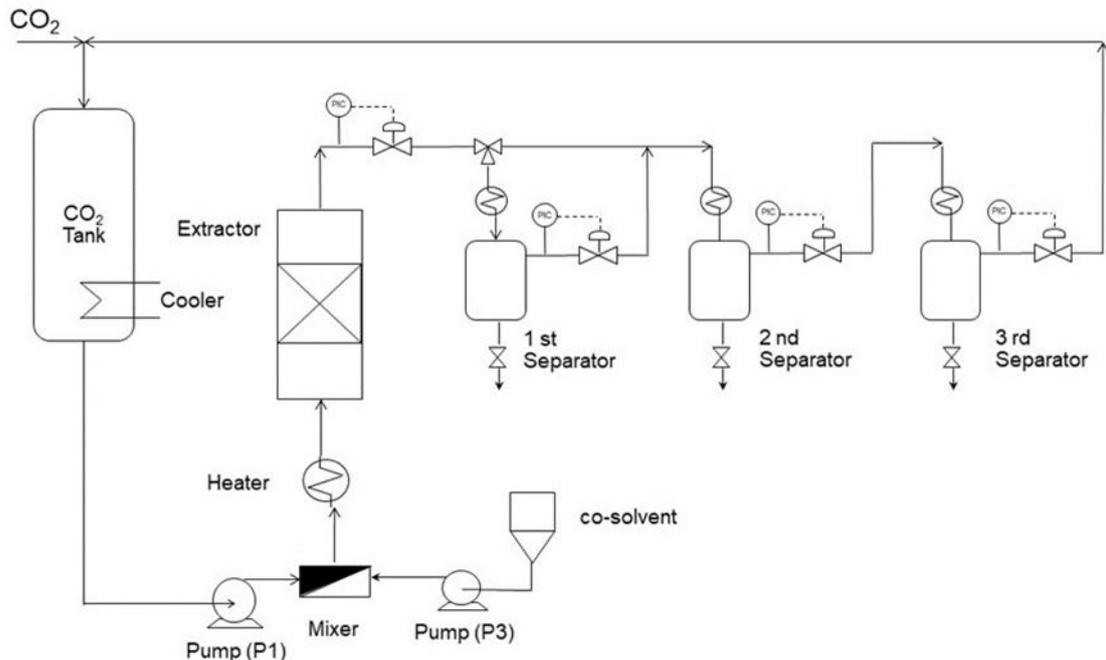
Figure 1: Block diagram of the Luwar CO<sub>2</sub>-SFE plant
