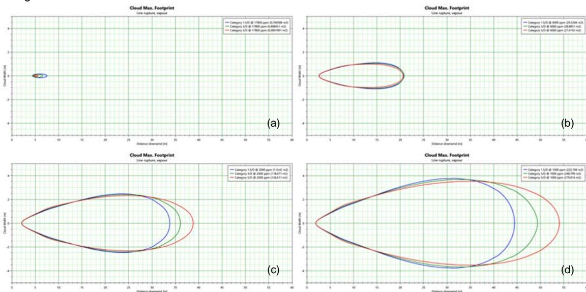
Figure 5: CO<sub>2</sub> iso-concentrations as a function of distance downwind at different values of CO<sub>2</sub> concentration (17,800 ppm (a), 6,000 ppm (b), 2,000 ppm (c) and 1,000 ppm (d)) after the breakage of a pipe leaving the extractor (Category of atmospheric stability: D)
