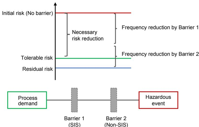
Figure 1: The risk reduction of frequency-reducing barriers against a specific process demand.
