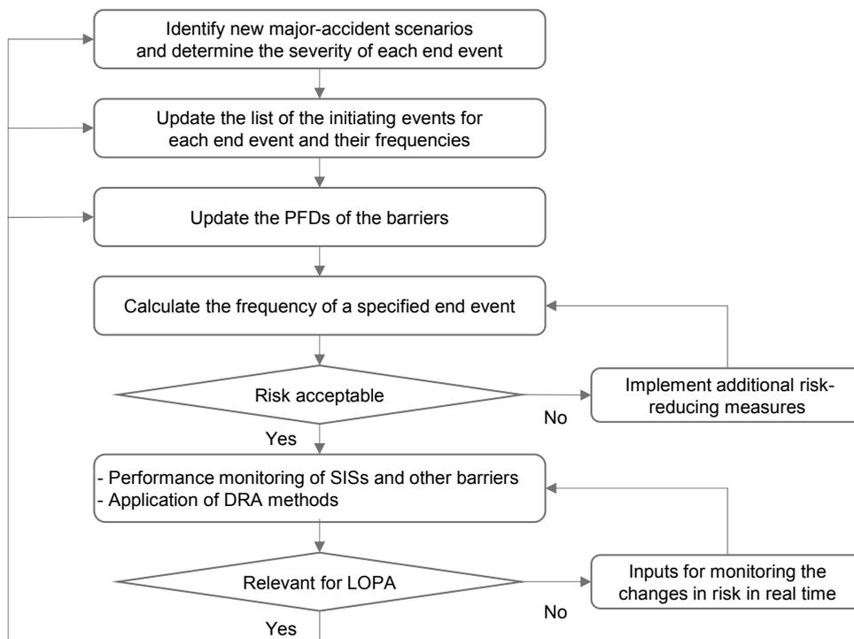
Figure 4: LOPA and performance monitoring of SISs during the operational phase
