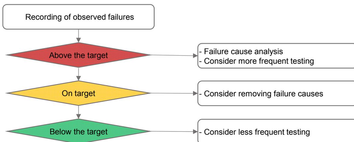
Figure 2: An example on how to use a performance indicator (e.g. observed number of DU failures) for verifying SIL requirements in the operational phase. Adapted from (Hauge et al., 2008).
