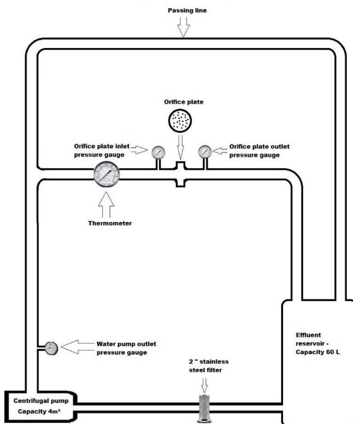
Figure 1: Diagram of the hydrodynamic cavitation equipment
