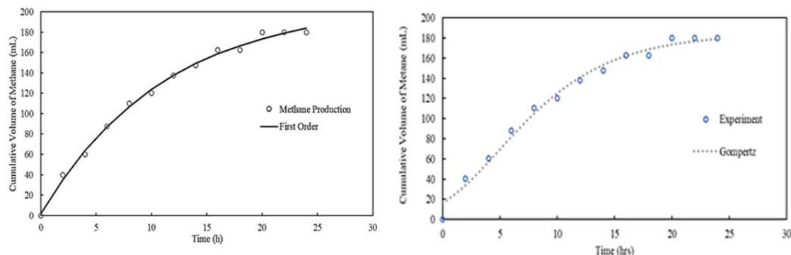
Figure 3: Kinetics Models Fitting for (a) First Order Kinetic Model (b) simplified Gompertz Model
