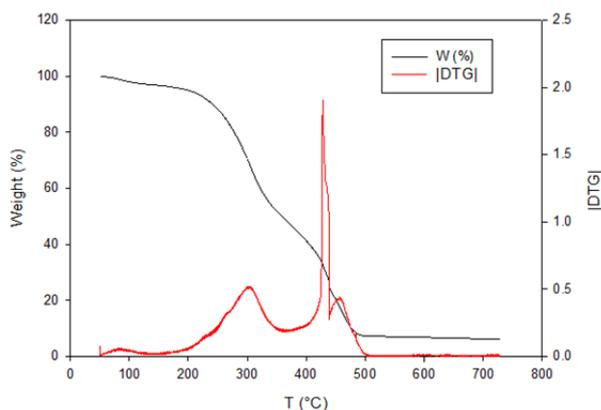
Figure 4: Weight percentage and DTG as a function of temperature, TG/DSC analysis, 10 °C/min, airflow
