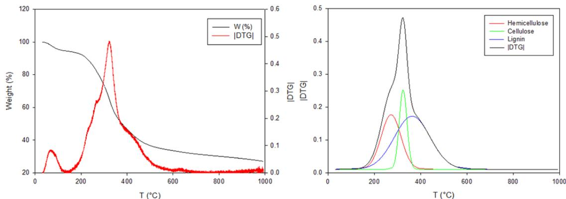
Figure 3: Weight percentage and DTG curves as a function of temperature, TG/DSC analysis, 10 °C/min, N<sub>2</sub> flow (left), and deconvolution through Fraser-Suzuki equation of DTG curve (right).
