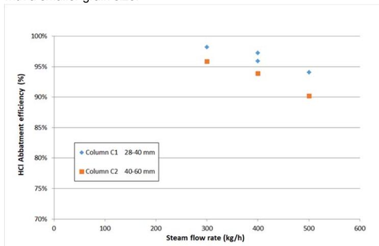
Figure 3: Abatement efficiency for different grain size for various flow rate at constant pressure.
