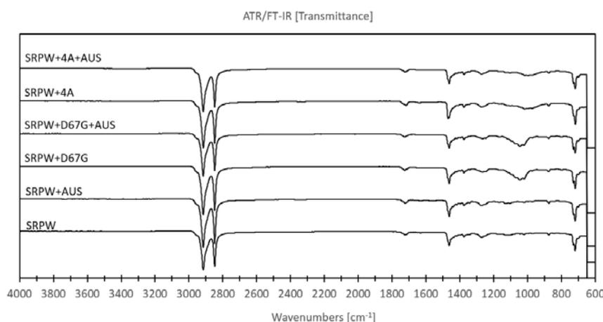
*Figure 4: ATR/FT-IR spectrum of SRPW-based mixtures additivated with D67G and zeolite 4A, with and without compatibilizer addition.*
