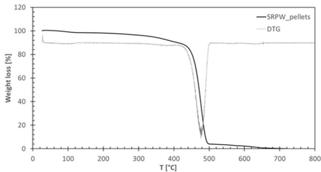
Figure 2: Thermogravimetric plot of SRPW in form of pellets.
