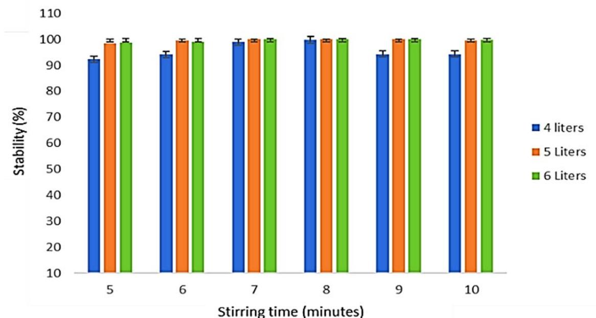
Figure 5: Stability percentages of agitation times in relation to the volumes investigated in the production process of Biodetergent, after 96 hours of rest
