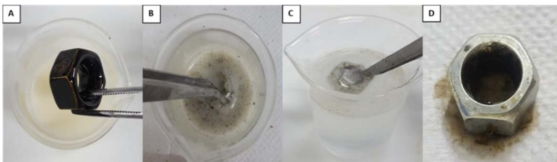
Figure 7: Illustration of the removal of OCB1 oil by Biodetergent on a metallic surface. (A) metal part impregnated with OCB1 oil. (B) removal of OCB1 after immersion in the formulation. (C) removal of destabilized oil residues in the part after immersion in water. (D) Removing oil on the finished metal surface
