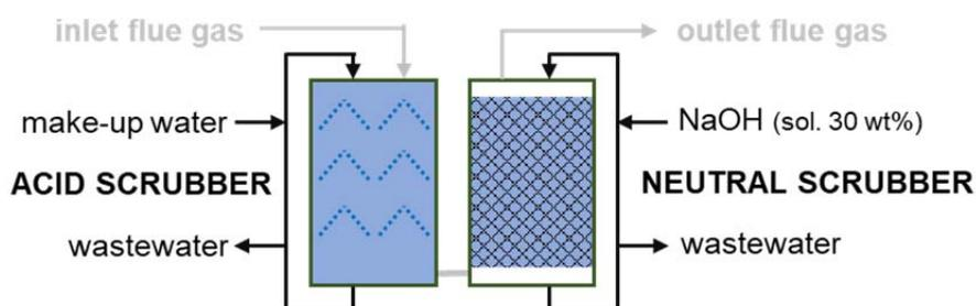
Figure 1: Reference scheme for the wet scrubbing system.
