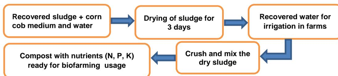
Figure 3: Schematic diagram for nutrients and water recovery for biofarming usage.
