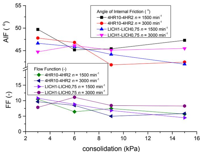
Figure 8: Flow properties of the product obtained at different parameters of the matrix and rotor speed
