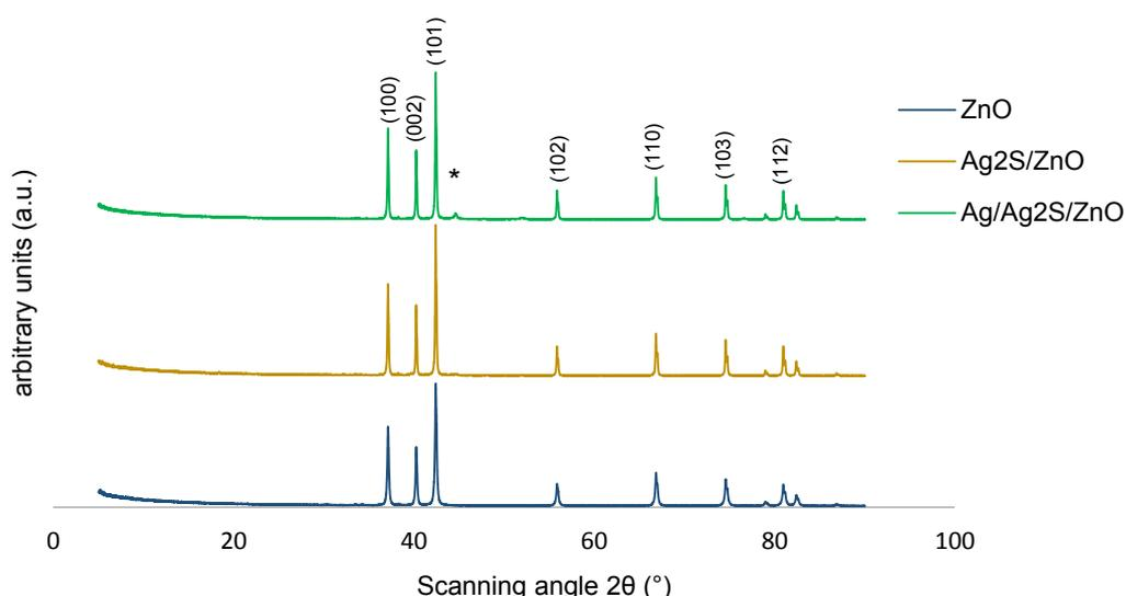
Figure 1: XRD pattern of crystalline ZnO, Ag<sub>2</sub>S/ZnO and Ag/Ag<sub>2</sub>S/ZnO
