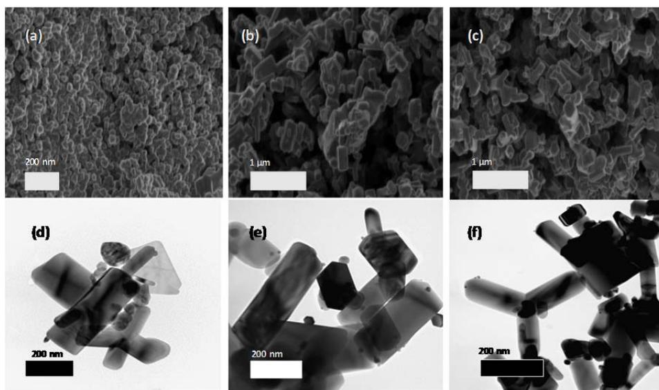
Figure 2: SEM (a), (b), (c) and TEM (d), (e), (f) images of ZnO, Ag<sub>2</sub>S/ZnO and Ag/Ag<sub>2</sub>S/ZnO
