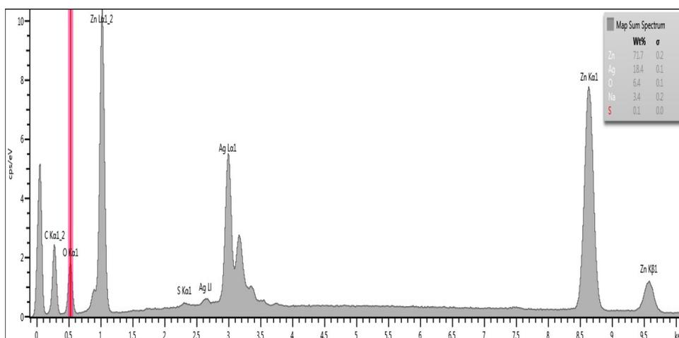
Figure 3: EDX spectra of ternary Ag/Ag<sub>2</sub>S/ZnO nanopowder.
