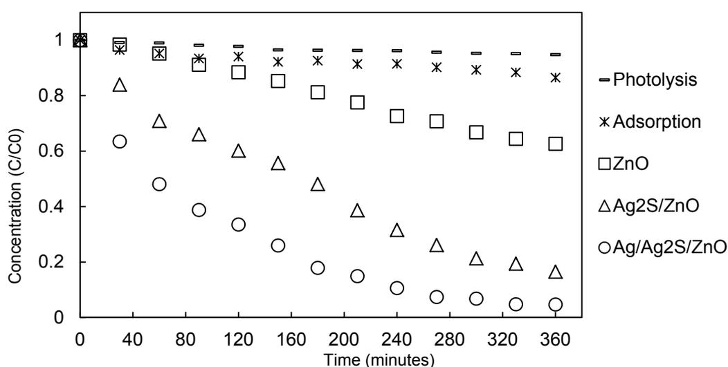
Figure 4: Phenol degradation with time under visible light irradiation
