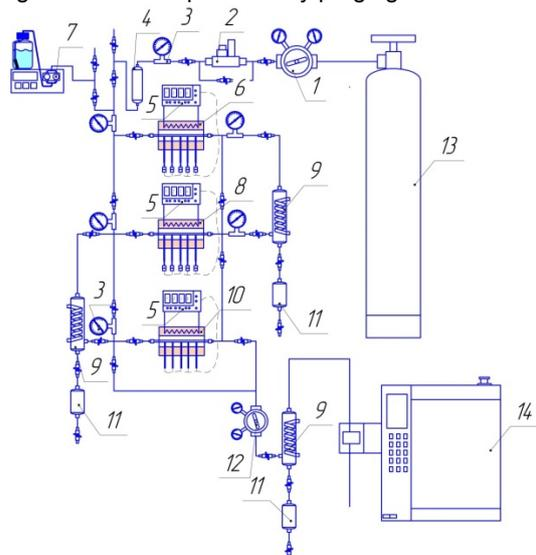
Figure 1. Reaction set up for methanol to hydrocarbons catalytic transformation:
