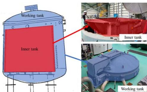
Figure 2: VPI tank configuration overview
