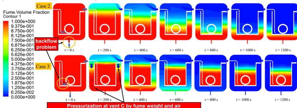
Figure 6: Changes in the fume contour for cases 2 and 3 according to time
