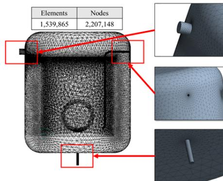
Figure 4: Mesh configuration of the geometry
