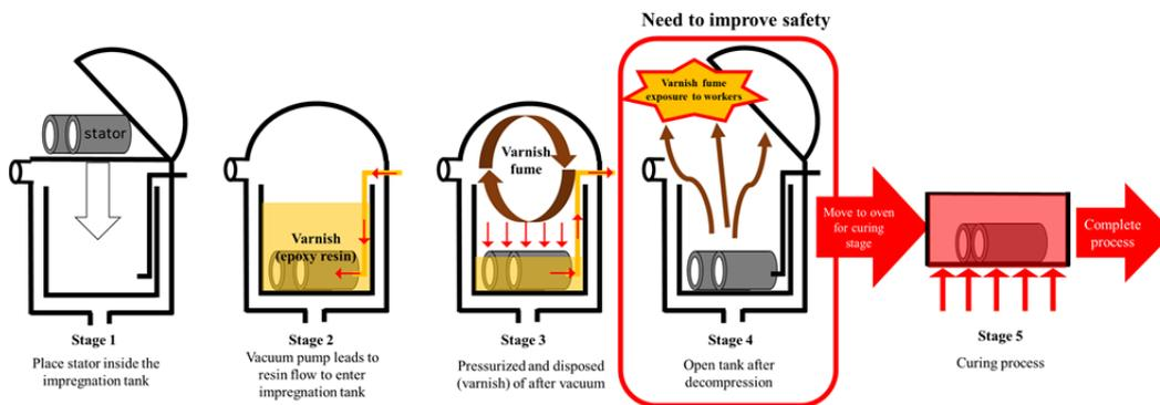
Figure 1: Schematic diagram of the VPI process
