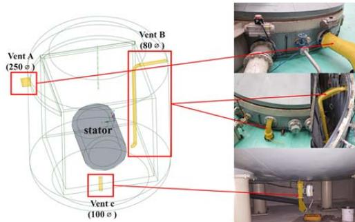
Figure 3: Geometry of VPI tank for CFD
