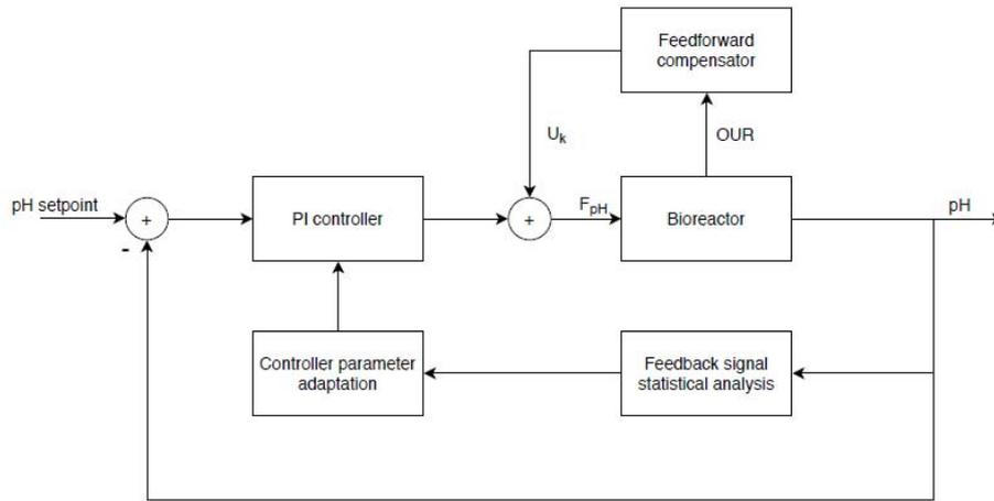
Figure 3: Block-diagram of the adaptive pH control system
