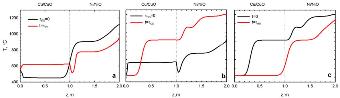
Figure 1: Spatial temperature profiles at several time instants during RS (a), OS (b) and HR (c)
