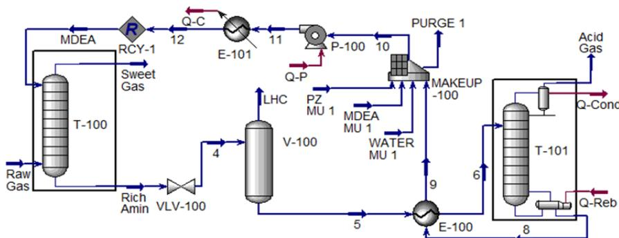
Figure 3: Process flow diagram for Alestiklal sweetening unit by Aspen HYSYS software.
