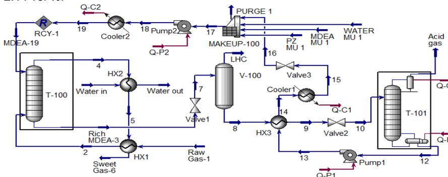
Figure 1: Process flow diagram for Mellitah sweetening unit by Aspen HYSYS software
