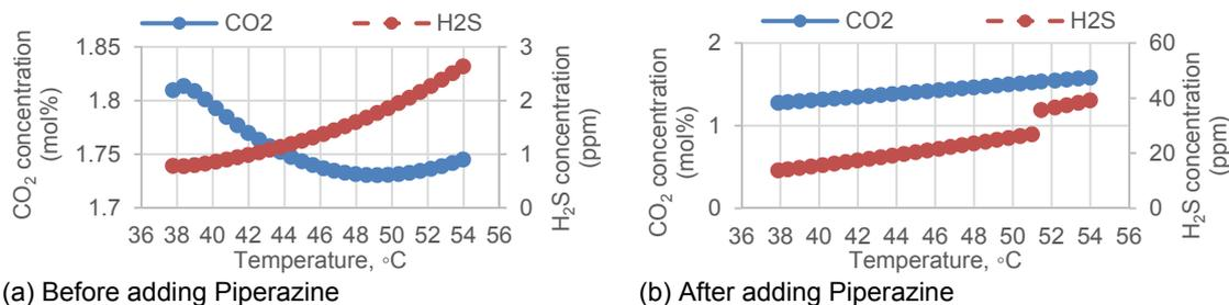
Figure 5: Effect of lean solvent temperature on sweet gas composition.
