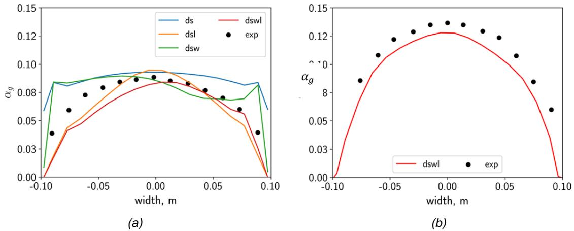
Figure 2: Square column with gas-liquid flow, (a) Impact of interfacial forces on the local gas hold-up at height  $z/L = 3$  and superficial gas velocity 0.02 m/s (gas-liquid flow). Legend reports the enabled forces for each line: drag (d), swarm correction of the drag (s), lift (l) and wall lubrication (w). (b) Local gas hold-up at height  $z/L = 3$  and superficial gas velocity 0.034 m/s.
