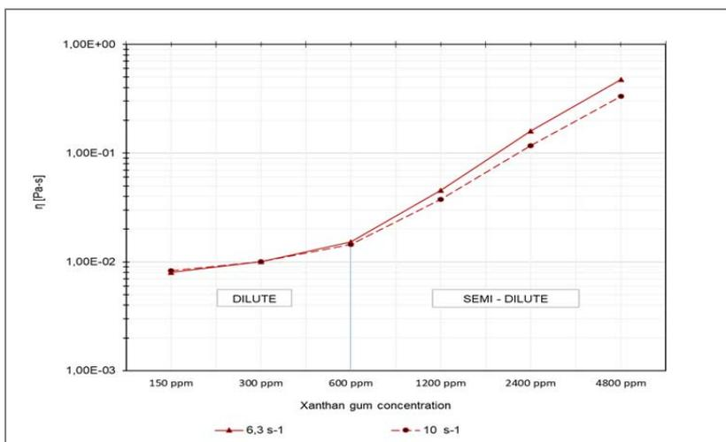
Figure 3: Dilution curve of xanthan gum with 3% NaCl. Shear rates of 6.31 s<sup>-1</sup> and 10 s<sup>-1</sup>.
