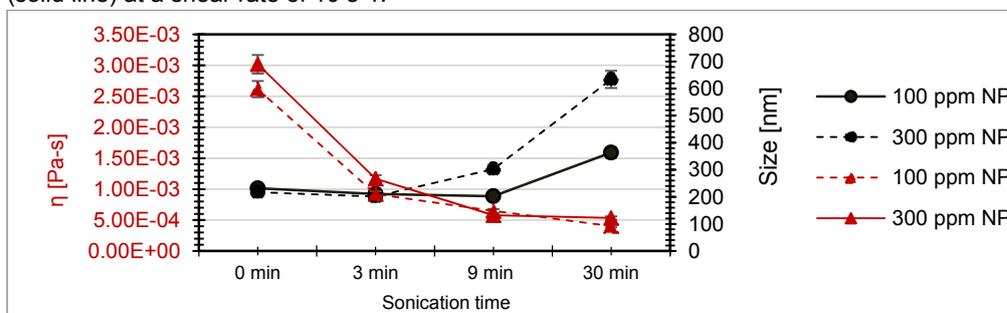
Figure 4: Viscosity at 10 s<sup>-1</sup> and particle size of NP suspensions as a function of sonication duration. Left axis: viscosity  $\eta$  (red); Right axis: nanoparticles size (black).
