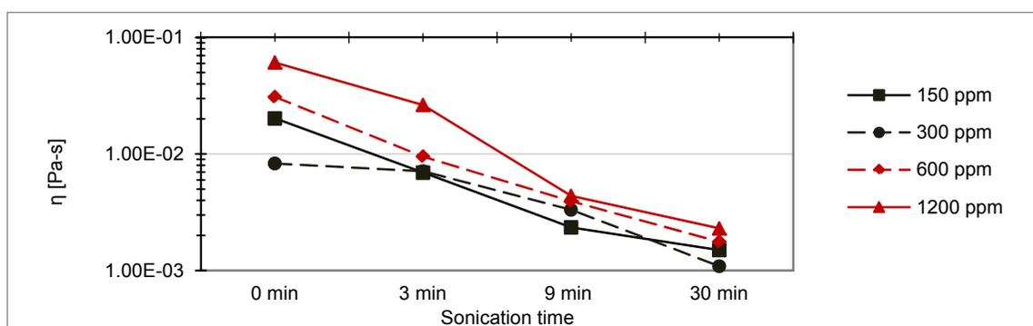
Figure 1: Effect of sonication on viscosity curves for xanthan gum solutions at a shear rate of 10 s<sup>-1</sup>
