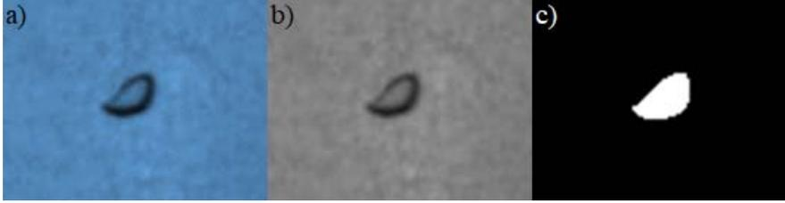
Figure 2: Selected stages of image processing; a) colour image, b) grayscale image, c) binary image
