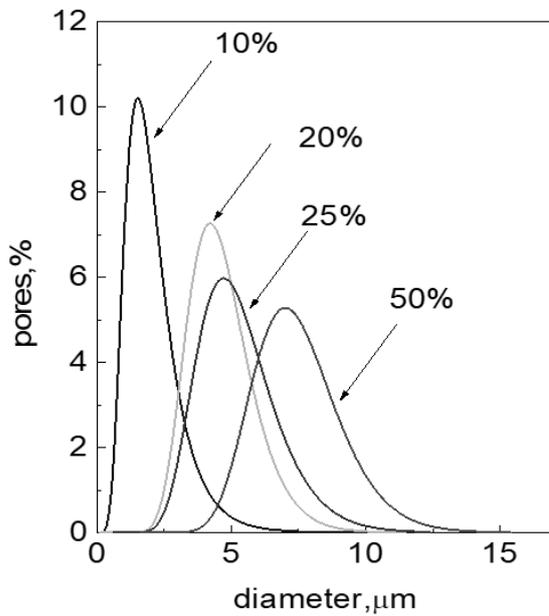
Figure 3. Pore size distribution of PMMA porous structures obtained at 200 bar and 35°C and at different polymer concentration.
