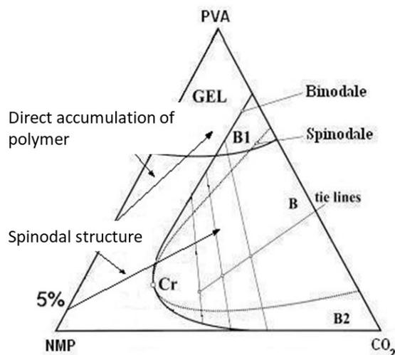
Figure 5: Qualitative ternary diagram: PVA-NMP- $\text{CO}_2$ .
