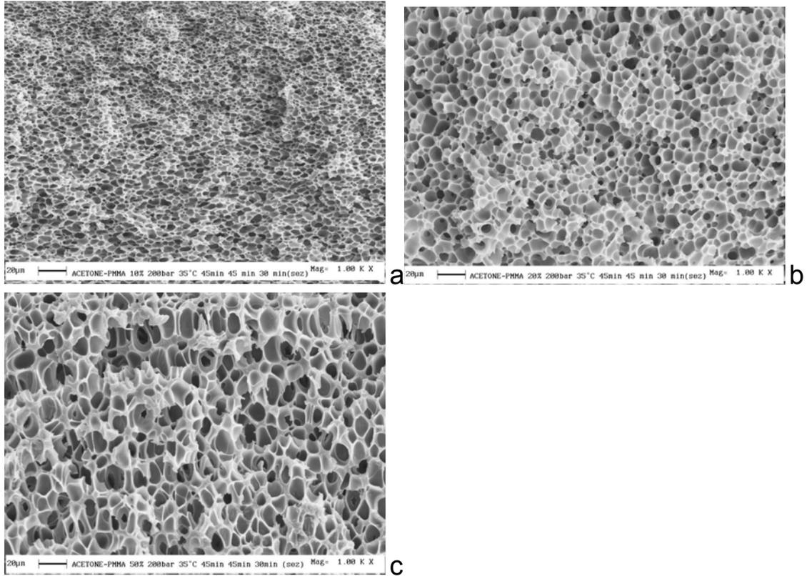
Figure 2. SEM images of PMMA internal section obtained at 200 bar and 35°C, at different polymer concentration: a) 10% w/w, b) 20% w/w, c) 50% w/w (scale bars = 20  $\mu\text{m}$ ).
