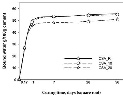
Figure 4. Bound water as determined up to 56 days of hydration (normalized to 100g of anhydrous cement) for CSA\_R, CSA\_10 and CSA\_20 plotted against curing time.
