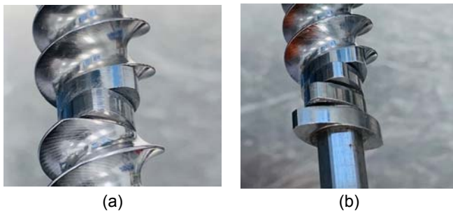
Figure 4: Kneading element configuration; (a) 2 KB and (b) 4 KB.
