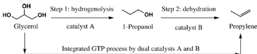
Figure 2: Catalytic conversion of glycerol to propylene
