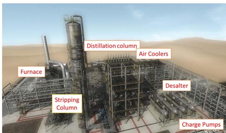
Figure 1: Virtual Crude Distillation Unit overview with the indication of the main units.
