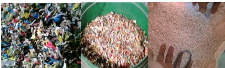
Figure 1: Shredded waste plastic (PE, mixed plastic, and PS) from left to right.
