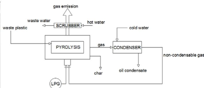
Figure 2: Pyrolyzer and the pyrolysis process.
