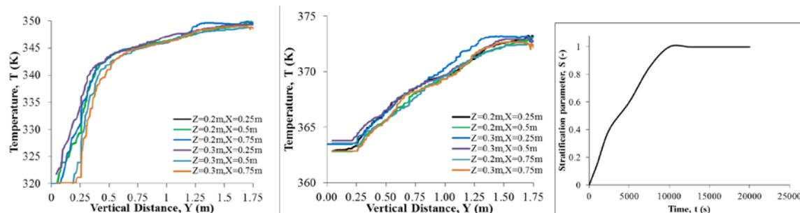
Figure 5 Spatial and temporal temperature variation. (A) and (B) represent axial temperature variation for two time instances  $t = 3,000$  seconds and  $t = 20,000$  seconds respectively and (C) Amount of stratification taking place quantified by Stratification parameter.
