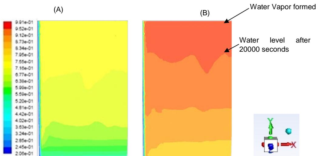
Figure 4: Volume fraction contours for the geometry for an initial height to 1.75 m and heat flux of 75 kW at  $z=0.2$  m (A)  $t = 3000$  s (B)  $t = 20000$  s
