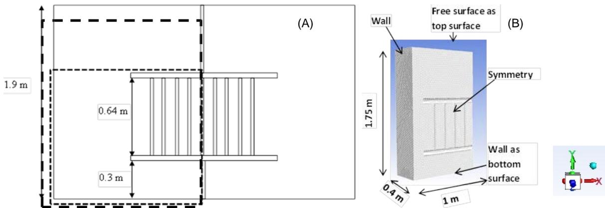
Figure 1: (A) Details of geometry used for simulations. Small dotted line represents the domain for simulations with initial height of 0.83 m and large dotted line represents domain for simulations with initial height of 0.83 m (B) Typical mesh used for simulations
