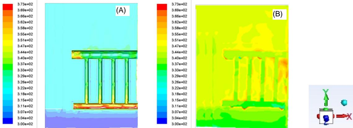
Figure 3: Temperature contours for the geometry for an initial height to 1.75 m and heat flux of 75 kW at symmetry plane  $z=0.01$  m (A)  $t = 1000$  s (B)  $t = 3000$  s
