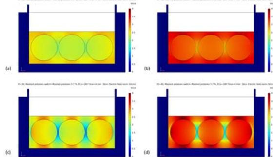
Figure 3. Electric field at 4min. APG=3 V/cm (a, c) and 4 V/cm (b, d), MP29 (a, b) MP57 (c, d),  $h=5 \text{ W}/(\text{m}^2 \text{ K})$
