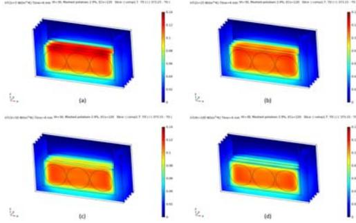
Figure 2. Slice plot of temperature after 4min, APG = 3 V/cm, MP29, (a)  $5 \text{ W}/(\text{m}^2 \text{ K})$ , (b)  $25 \text{ W}/(\text{m}^2 \text{ K})$ , (c)  $50 \text{ W}/(\text{m}^2 \text{ K})$  and (d)  $100 \text{ W}/(\text{m}^2 \text{ K})$
