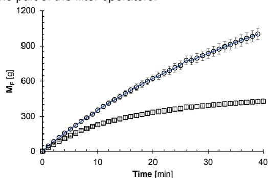
Figure 3: Time course of the mass of filtrate ( $M_F$ ) from a porous filter cake made of FC and a mixture of DE powders DIA1 and DIA2 (weight ratio of 1:9  $g.g^{-1}$ ) of lot A (O) or B (□) when feeding BP1 at 20 °C.
