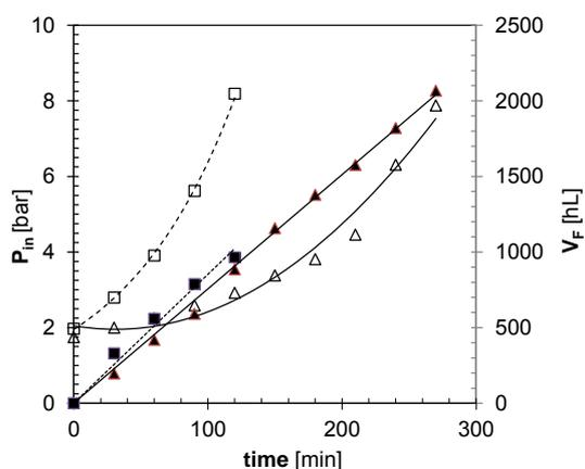
Figure 2: Time course of the operating pressure ( $P_{in}$ : open symbols) and volume of filtrate collected ( $V_F$ : closed symbols) from an industrial DE filter during the clarification of rough beer samples BP1 ( $\square, \blacksquare$ ) and BP2 ( $\triangle, \blacktriangle$ ).
