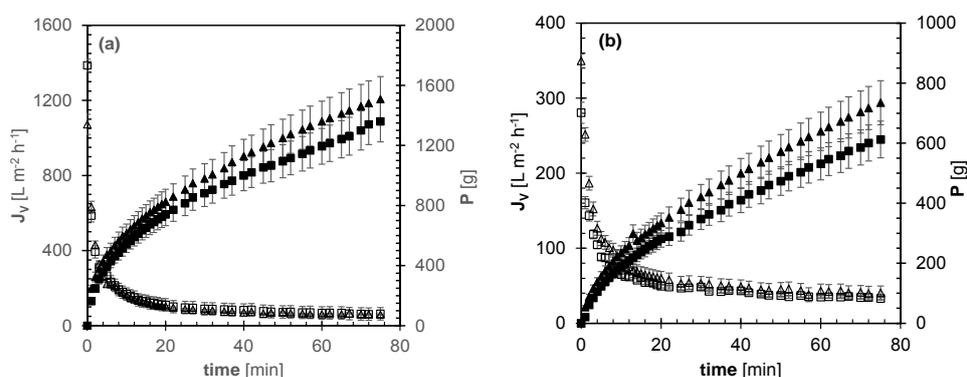
Figure 4: Time course of the instantaneous permeation flux ( $J_v$ , open symbols) and permeate mass (P, closed symbols) recovered during the CFMF of rough beer samples BP1 (□, ■) and BP2 (△, ▲) either pre-centrifuged at  $T=10$  °C (a) or used as such at  $T=1.5$  °C (b),  $TMP=3.75$  bar, and  $v_s=6$   $m.s^{-1}$ .
