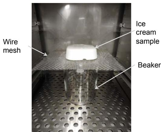
Figure 3: Experimental setup for melting test
