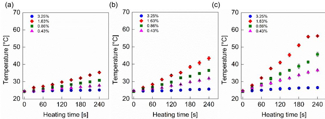
Figure 2: Heating rates of the basil-based sauce samples at the different  $\Delta V/L$ : (a) 3.12 V/cm, (b) 4.16 V/cm and (c) 5.20 V/cm.
