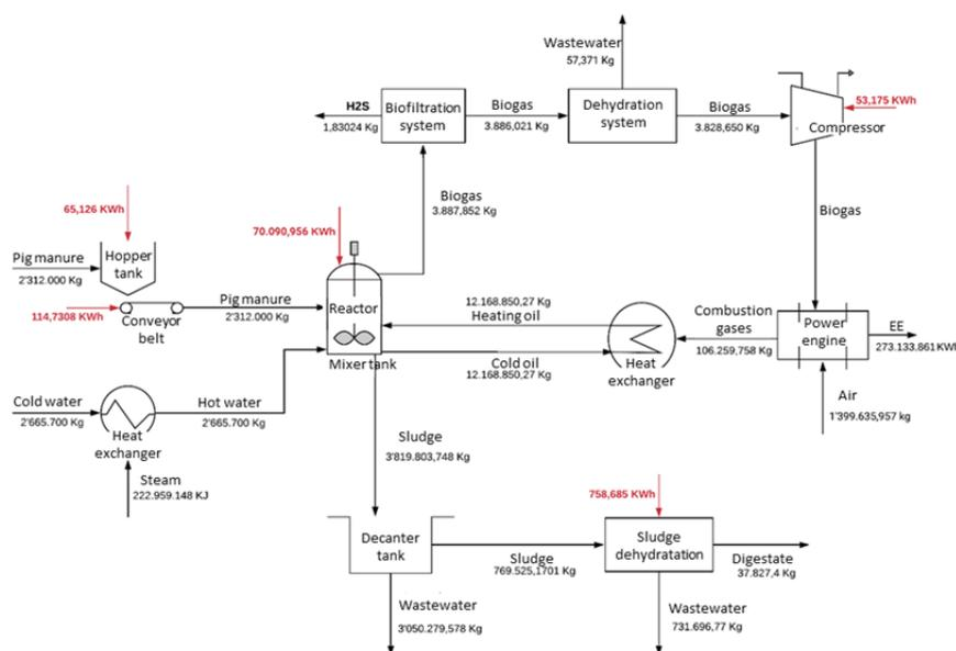
Figure 1: Diagram of AD process for PM
