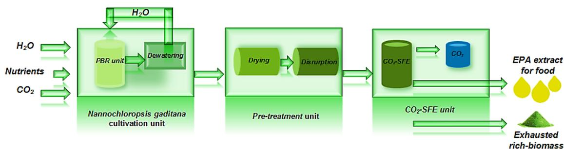
Figure 1: EPA and exhausted biomass production from *Nannochloropsis gaditana* in VALUMAG plant
