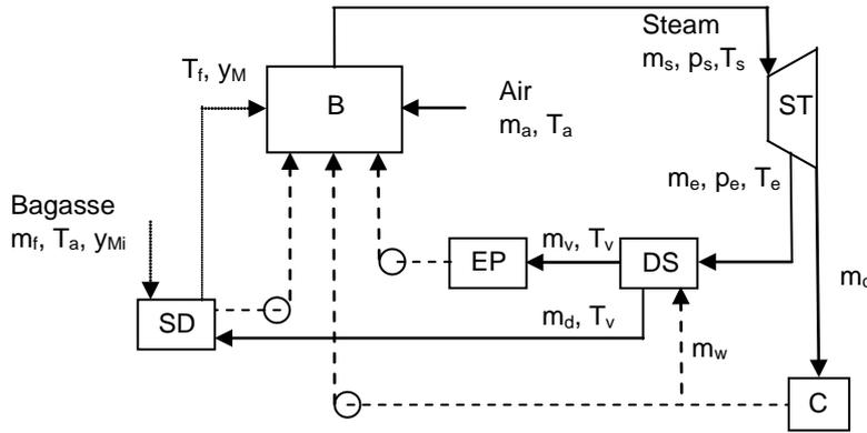
Figure 2: Cogeneration system in cane sugar industry.
