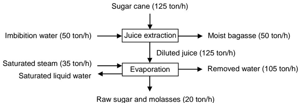
Figure 1: Mass balances in raw sugar manufacturing process.
