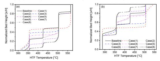
Figure 3: HTF axial temperature distribution over height after 300 min for (a) Charge and (b) Discharge cycles
