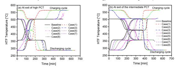
Figure 4: HTF temperature at the exit of high and intermediate PCM
