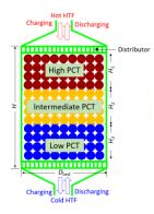
Figure 1: Schematic representation of the TES tank system
