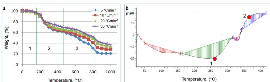
Figure 1: **a** TGA analyzes carried out in an argon atmosphere, the process of pyrolysis of rice husks, **b** thermal effects of decomposition of hemicellulose and cellulose for  $\beta = 5\text{ }^{\circ}\text{C/min}$ .
