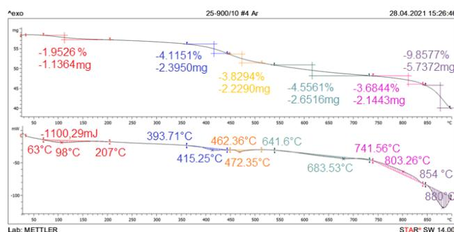
Figure 2: Graphical images of DSC and TGA analyzes carried out in an argon atmosphere, reduction of tin oxide using coals from the Shubarkol deposit
