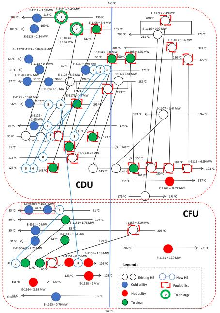
Figure 2: Grid diagram of the preheat trains of CDU (upper) and CFU (lower)
