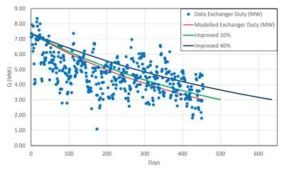
Figure 4: Performance of a heat exchanger and its estimated improved performance by 10 % and 40 %
