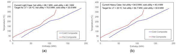
Figure 1: Composite Curve for current (a) light and (b) heavy cases
