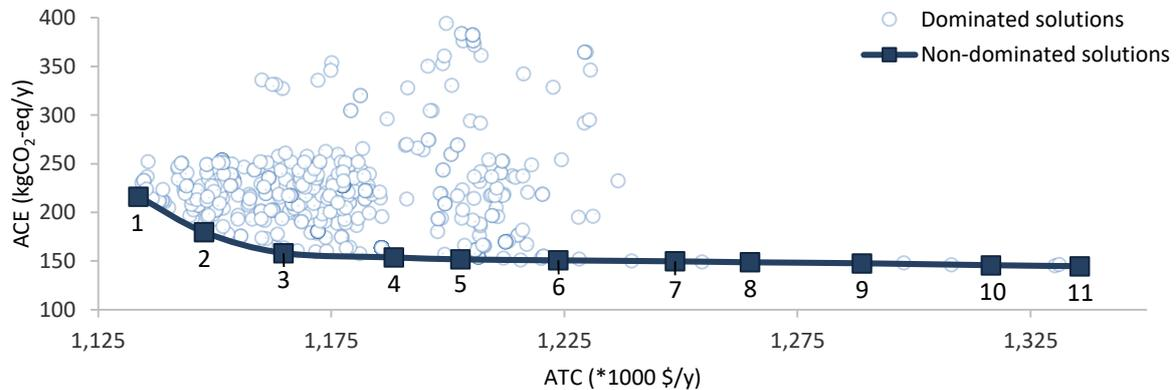
Figure 3: Pareto optimal set with multi-objective optimisation with EES, TES and HES.
