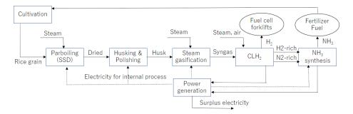
Figure 1: Schematic diagram of the proposed integrated system.
