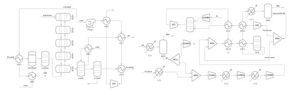
Figure 3: Process flow diagram of gasification, syngas chemical looping (CLH<sub>2</sub>).
