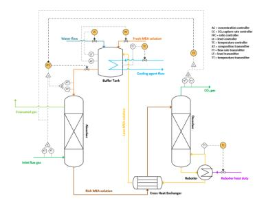
Figure 1: Process diagram and structure of the control system for the post-combustion CO<sub>2</sub> carbon capture plant
