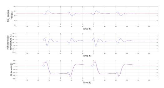
Figure 3: Carbon capture rate, reboiler temperature and molar ratio of MEA and CO<sub>2</sub> controlled variables (red line for the setpoint and blue line for controlled variable)
