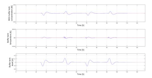
Figure 4: Concentration of MEA, temperature and level controlled variables in the buffer tank (red line for the setpoint and blue line for controlled variable)
