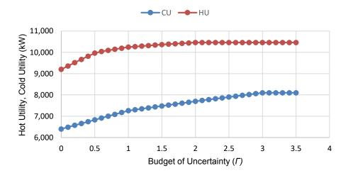
Figure 4: Graphical representation of varying budget parameters on hot and cold utilities
