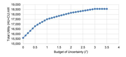
Figure 3: Graphical representation of varying budget parameters on total utility consumption due to uncertainty in inlet temp. of streams
