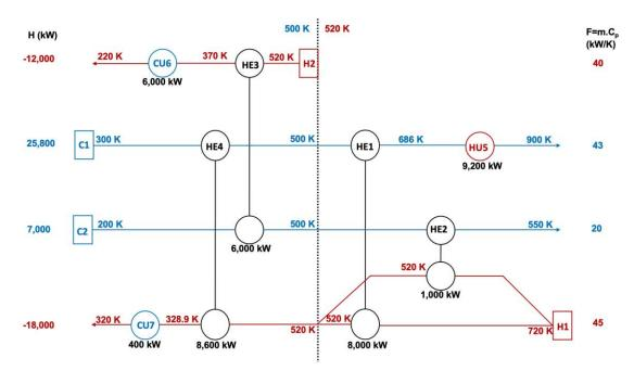
Figure 2: Grid Diagram of HEN for the deterministic value with no uncertainty
