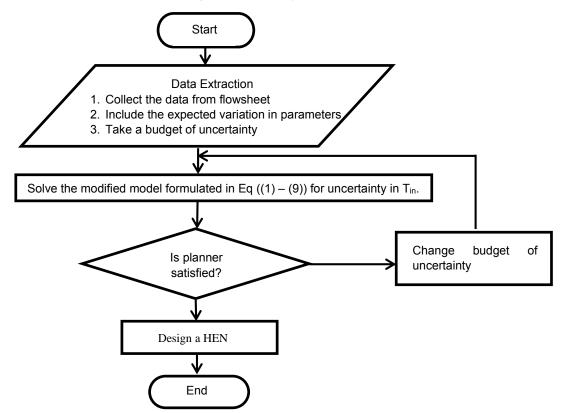
Figure 1: Flowchart for HEN design with parametric uncertainty
